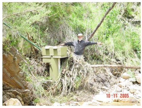
Figure 3 First Creek Gauging Station Above the Waterfall - Author Showing Peak Water Level
